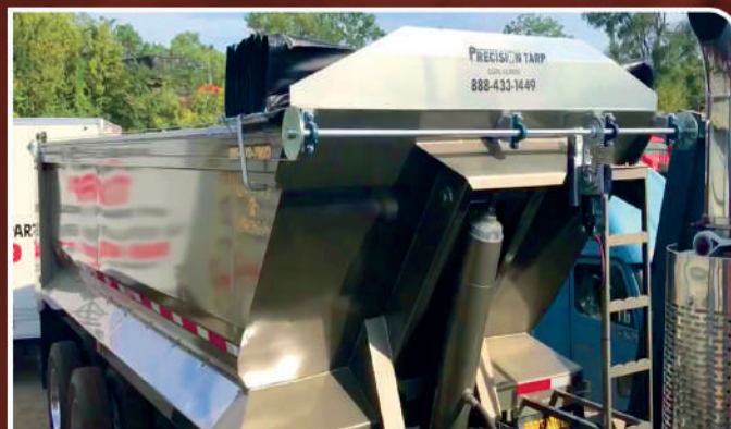
Heavy Duty Cable System w/ Electric motor installed on a Coras Trailer
