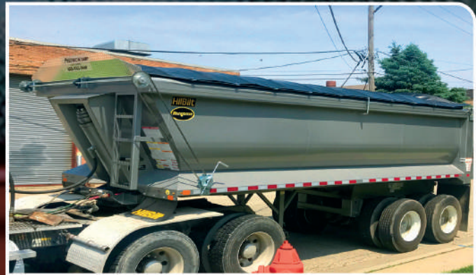
Heavy Duty Cable System installed on a Hilbilt Trailer
