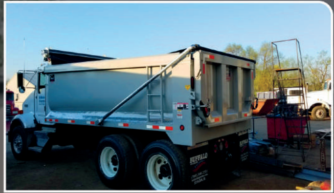
4 Spring External Mount System installed on a Buffalo Trailer
