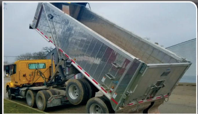
15 Coil Underbody Mount installed on an East Trailer
