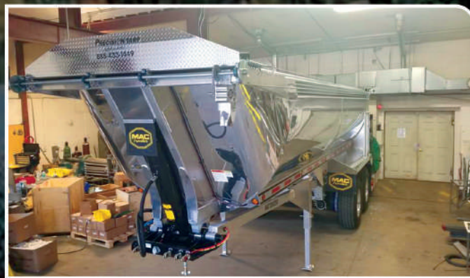
Heavy Duty Cable System w/ Electric motor installed on a Mac Trailer
